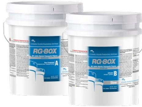
Two-component, high gloss, UV stable polyaspartic polyurea floor coating is formulated for use in industrial and commercial facilities and is designed to be used as a clear finish over broadcast floors. Suitable for both interior and exterior applications. RG-80x can be tinted to finish color.
